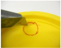
**Step 3:** Use a utility knife to cut out the inside of the circle that was just traced. Be sure to cut along the inside of the trace mark.
