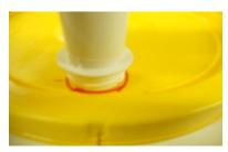
**Step 2**: Trace around the threaded section of the Pump on the top of the pail lid
